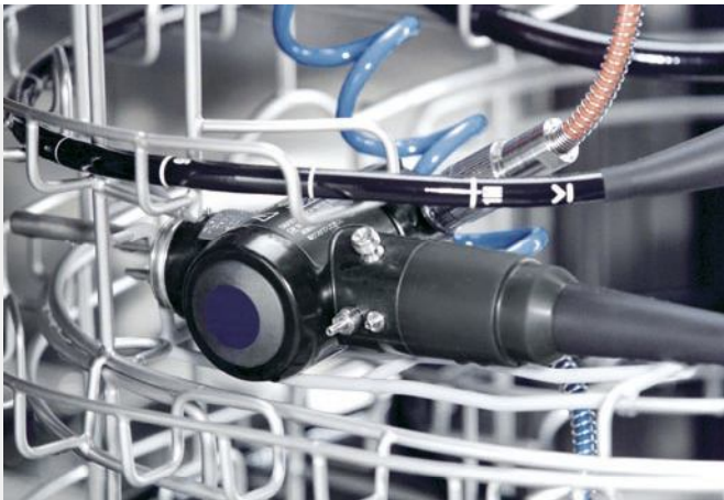
Endoscopes are automatically identified via transponders.
