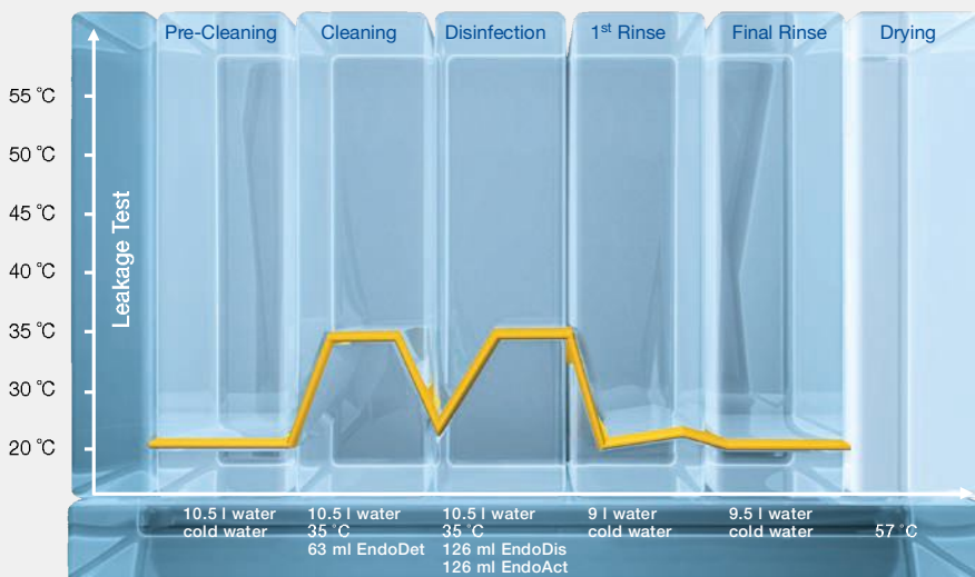
The PAA process works at 35 °C.
